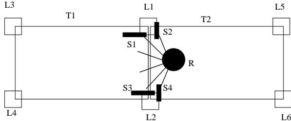
Figure 7: Typical ambiguous table scenario. Here the robot  $R$  has reported shapelets  $S1 - 4$  and inferred legs  $L1, 2$  unambiguously. But these legs are equally compatible with tables  $T1, 2$  having legs  $L3, 4$  and  $L5, 6$ . Exploring any of these four legs would remove the ambiguity about the tables.
