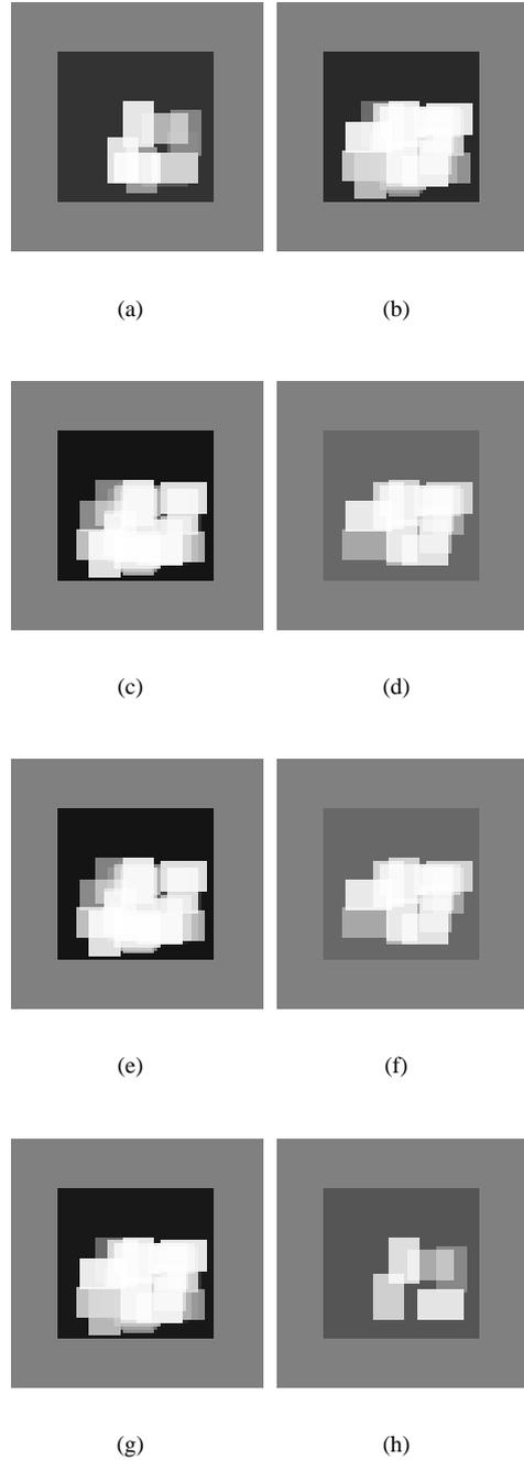
Figure 13: Examples of pairs (rows) of entropy maps. Each pair shows the table grid cell occupancy probabilities, conditioned on the presence (left) or absence (right) of a leg at some location in the arena. It can be seen that the entropy change is dominated by the shading of the background rather than the table distribution proper.
