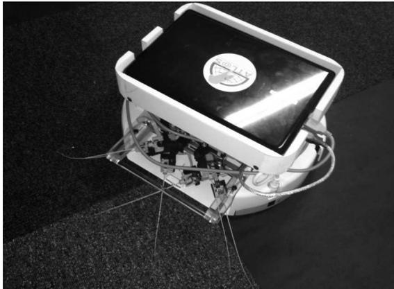
Figure 2: CrunchBot, a whiskered mobile robot platform.
