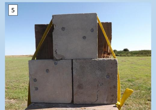
Figure 5: .22 caliber lead bullet impacts at the Caldicot rifle range
