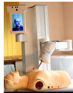
Fig. 2. The ReMeDi system on the site of the patient which shows the robot with an attached screen to display the doctor's face.
