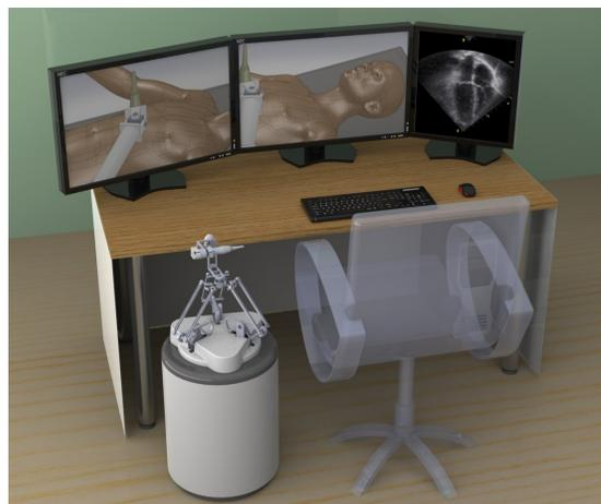
Fig. 1. Visualization of the ReMeDi system at the doctor's location: the doctor has communication interfaces to the patient and the assistant as well as a control console for the remote robot.
