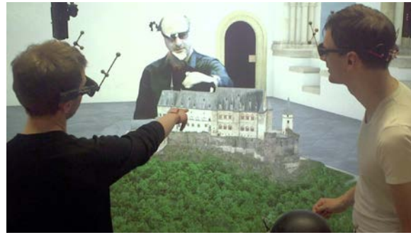
Figure 2. Collaborative wayfinding in a telepresence setting. The remote user is captured and represented as a 3D video avatar in the virtual environment. (Vianden Castle model courtesy of ArcTron 3D)
