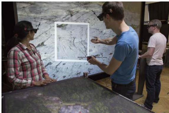
Figure 3. A large 3D powerwall (back) and a multitouch 3D tabletop (front) serve as independent multi-user 3D viewports into a shared virtual world. A virtual 3D display, or portal (center, with white frame), offers additional perspectives. The physical and virtual viewports serve for private interaction and group exchange. Their combination in a coherent workspace supports fluent transitions between tightly and loosely coupled cooperation. Here, a multi-scale 3D scan of prehistoric rock art and its environment (Valcamonica, Italy) is explored.
